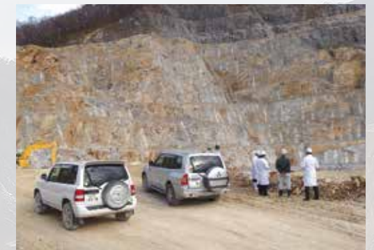
Limestone is mined and produced through the bench-cut mining method at an open-pit mine
