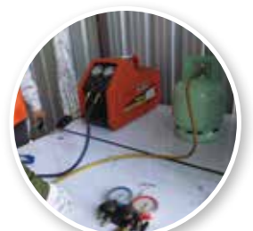
Fluorocarbon recovery system
